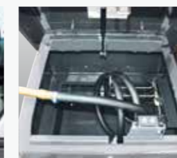
Electric fuel refilling pump
